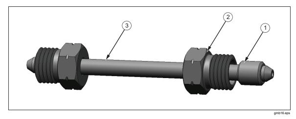
Figure 15. High Pressure Line
