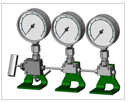
Figure 7. Gauges Ganged Together with a Valve
