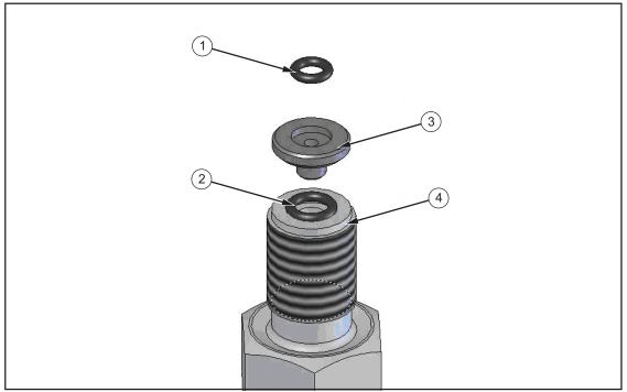
Figure 14. Test Port Insert
